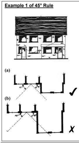
The second example is applicable if the dwellings are staggered. The extension shown on the plan encroaches across the 45° line. However, if the extension is single storey and below the 25° line (elevation (a)) then it would be in accordance with the 45° rule. However, if the proposal is two storey and it encroaches on the 25° line (elevation (b)) it becomes unacceptable.
